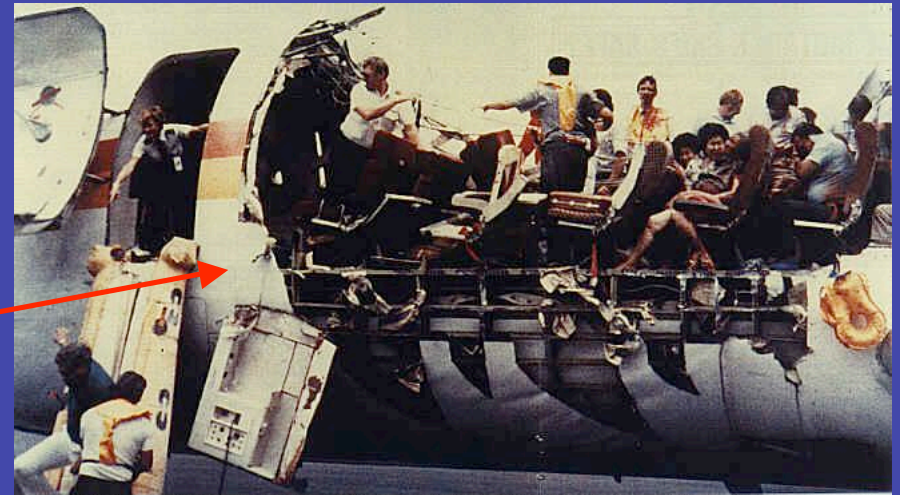
4-28-1988 After 89,090 flight cycles on a 737-200, metal fatigue lets the top go in flight.
